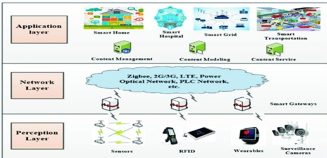
Fig. 13. Layers in IoT system [102]
