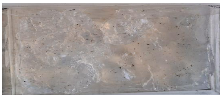
Fig. 8. Preparation of Hydrogel using chitosan extracted from crab shell and collagen from egg shell
