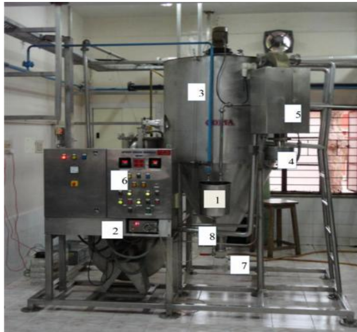
Fig. 5. Pilot scale spray dryer [25]
